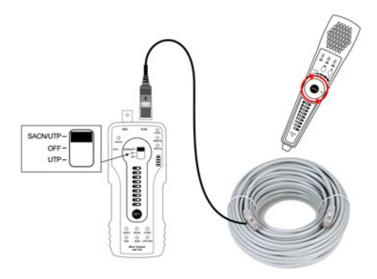
(2) Rotating the knob of receiver to adjust the sensitivity. When the cables are very close, can adjust to the small sensitivity to find the cable. Long press the "MUTE" key for silent mode. In this mode, the signal strength indicator light is used to trace the wire. When received the strongest signal, the eight indicator lights are on. Press "MUTE" again to exit MUTE mode.
