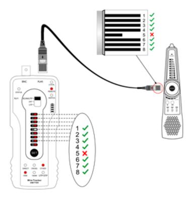
The mid-end of cable continuity detection: If the cable sequence detects that the cores of the cable are disconnected, and the local / remote cores are detected to be connected, indicating that the break point of the cable is in the middle position away from the ports on both sides.
